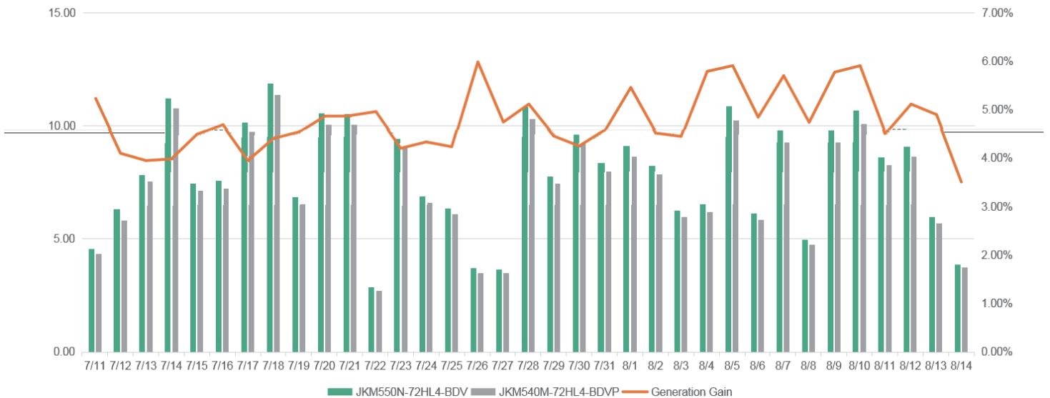
Figure 3. Daily energy yield on Zhangbei project
